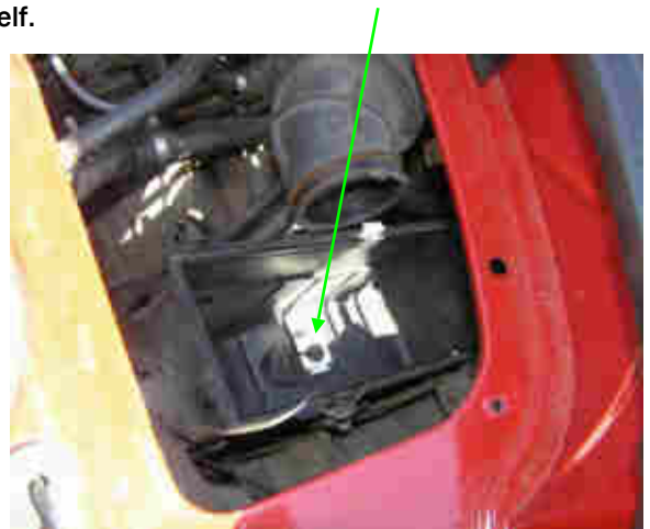
outside air temperature sensor mounted inside air filter box
